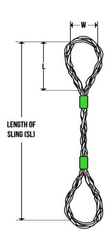
NOTE: RATED CAPACITIES OF CHOKER HITCHES APPLY WHEN THE ANGLEOF CHOKE IS GREATER THAN 120 DEGREES. 8-PART BRAIDS WITH CASINGS AND CHOKER HOOKS ALSO AVAILABLE.
